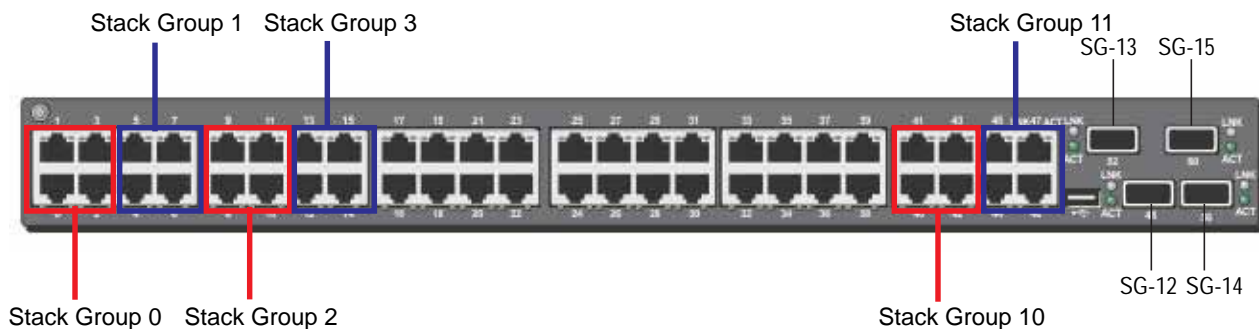
Figure 4-7. S4820T Stack-Group Assignment
